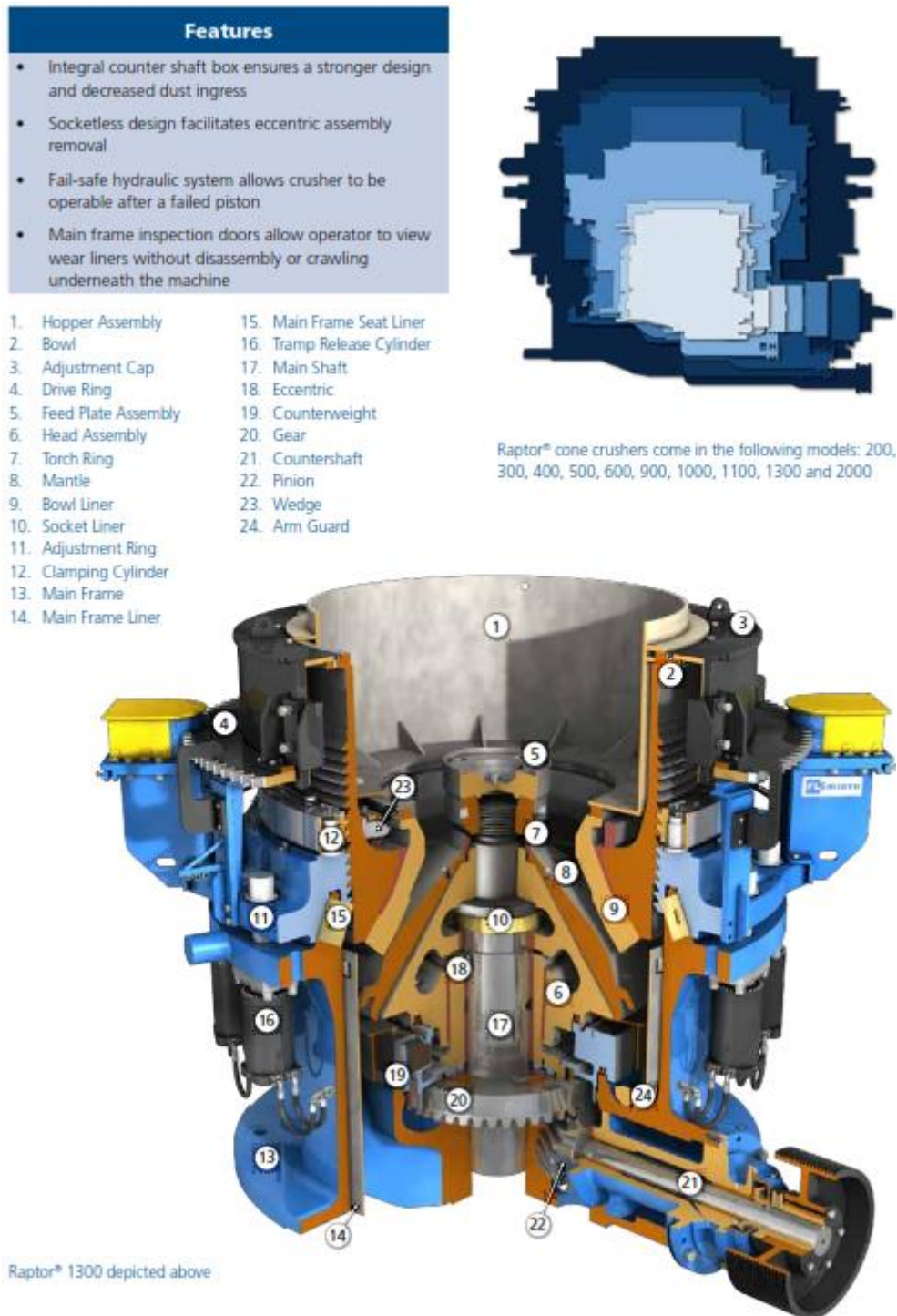
Figure 14-2: Secondary crusher schematic
